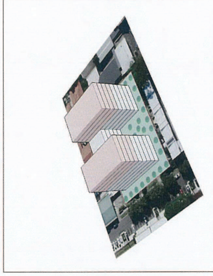
3. MASSING RELOCATED TO DEFINE CORNERS. SOLAR CORRIDOR TO MIDDLE OF BUILDING ENABLES SOLAR ACCESS TO ADJACENT TOWNHOUSES.
